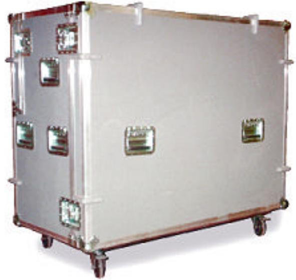
This case design has been developed to protect your display under the most extreme conditions of common carriers. It features a 3/8" ATA Style construction with ABS plastic outer surface, steel "ball" corner protection, spring loaded dish handles, .060 extruded aluminum double-channel edge protection and interlocking valance, shock absorbing rubber "bumpers", locking casters, and recessed keylockable twist latches.
